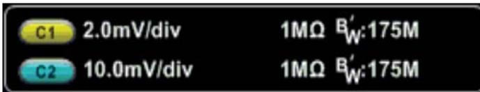
Figure 1. 2X Probe (CH1) and 10X Probe (CH2) Lowest System Vertical Sensitivity.
