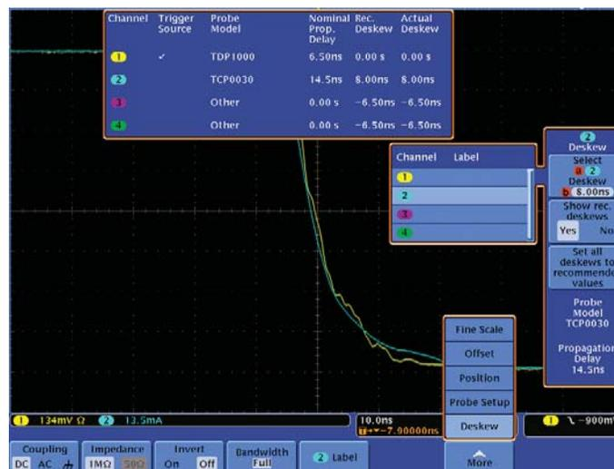
Figure 6 - Normal Correction of Timing Skew between Voltage and Current Probes
