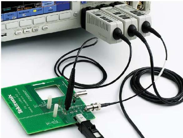
Figure 7 - Tektronix Deskew Pulse Generator and Deskew Fixture
