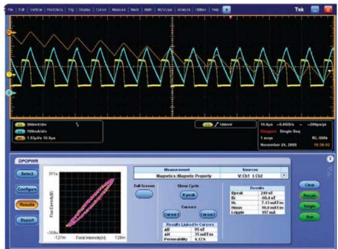
Figure 19. B-H plot for single winding inductor.
