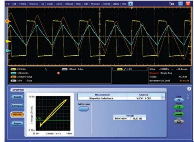
**Figure 14.** Inductance measurement results from DPOWPR application software.
