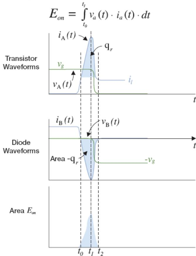
Figure 3. Turn-on Loss in a MOSFET with clamped inductive load.<sup>2</sup>
