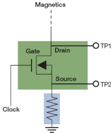
Figure 5. MOSFET switching device, showing measurement points.
