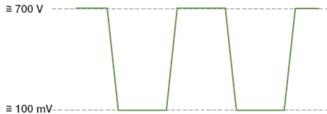
Figure 6. Typical signal of a switching device.
