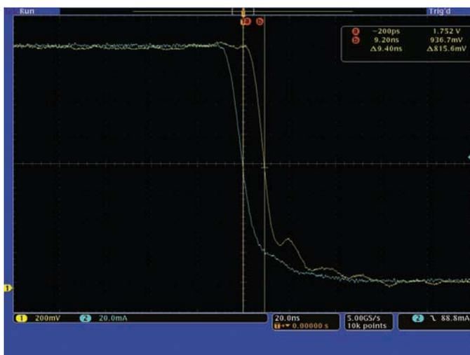
Figure 9. 9.4 ns skew between voltage and current signals.
