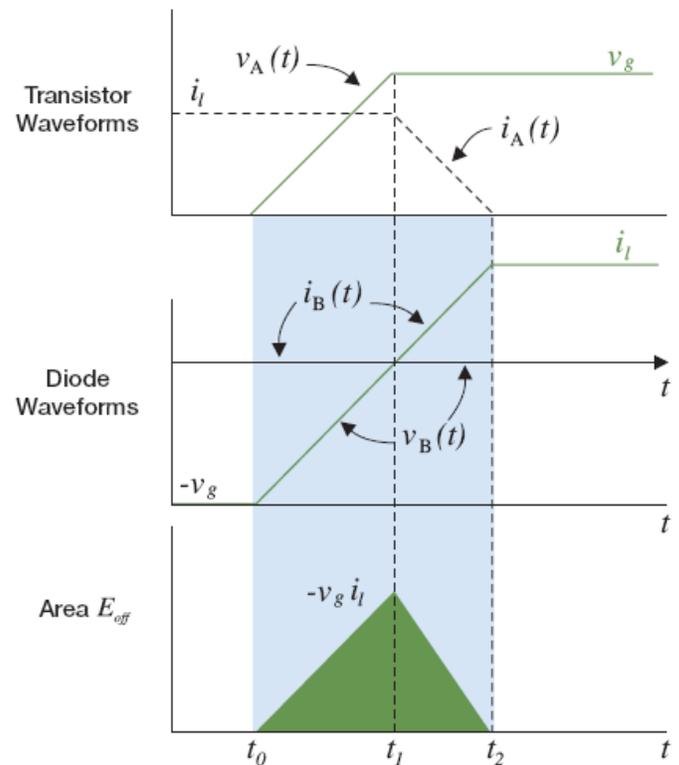
Figure 2. Calculation of Turn-off Loss.
