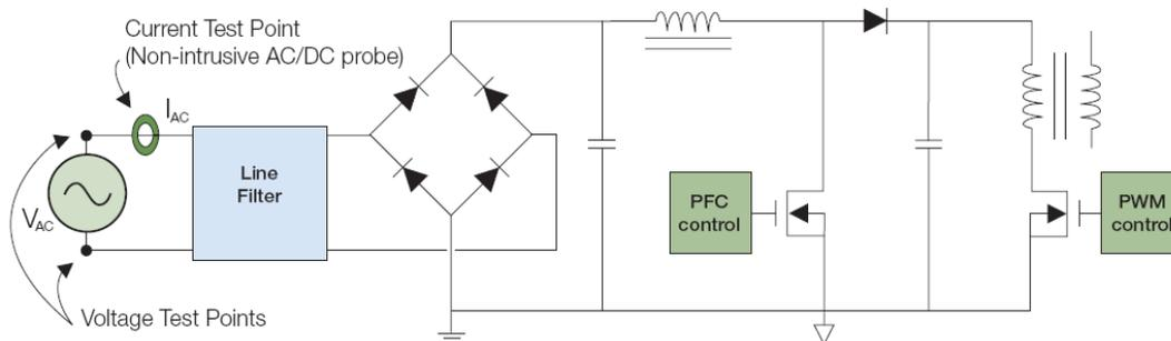
Figure 21. Simplified view of an SMPS power supply (primary side only) and its power quality measurement test points. Simultaneous input VAC and IAC readings are necessary for power quality measurements.
