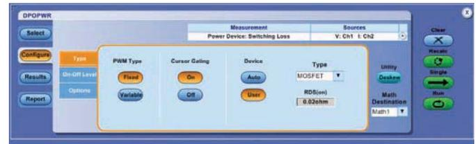
Figure 7. The DPOPWR input page allows the user to enter data sheet values for RDSON & VCEsat.
