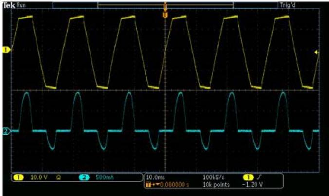
**Figure 25:** AC input voltage (yellow) and current (blue) waveforms. Figure 25 shows the voltage and current at the input to an AC-to-DC converter.
