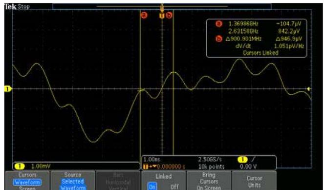
**Figure 14:** Cursor measurements identify noise as 900 MHz
