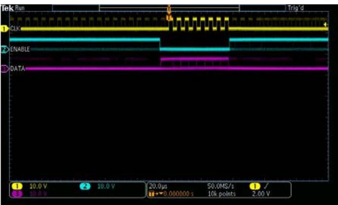
**Figure 8:** 3-wire SPI serial bus signals.
