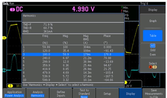
**Figure 30:** Tabular display of input current harmonics.
