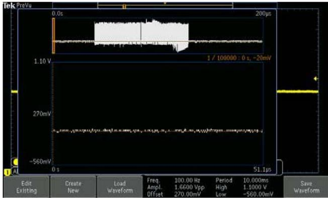
Figure 21: Noise-free CAN signal generated by the ARB.
