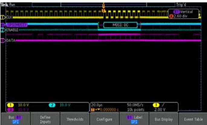
**Figure 9:** Automatic decode of the SPI serial bus.
