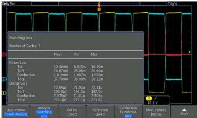
Figure 31: Switching Loss measurements.
