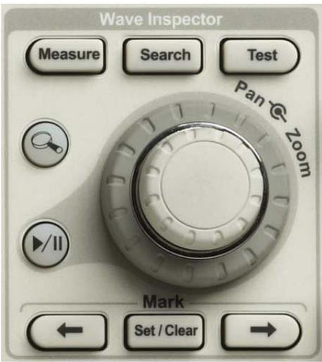
**Figure 5:** Front panel Wave Inspector controls
