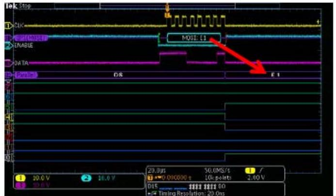
**Figure 10:** Digital channels and an 8-bit parallel bus added to the display.
