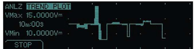
Figure 4 - TrendPlot display on the DMM4050/4040.
