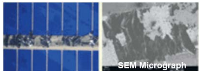
Figure 1: Conventional solder joint after peel-test using optical and SEM micrographs
