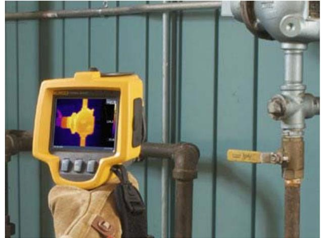
**If your facility uses a boiler, scan the steam lines to check for leaks, blockages, and failed traps.**
