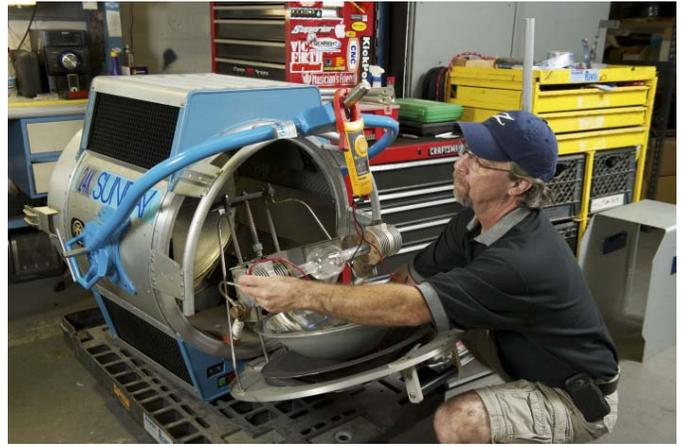
Phil Muskett of DADCO Power and Lights checks the continuity of an HMI light fixture's globe (lightbulb) with a Fluke 337 Clamp Meter. This is one of the largest light fixtures in the industry at 24,000 kilowatts.
