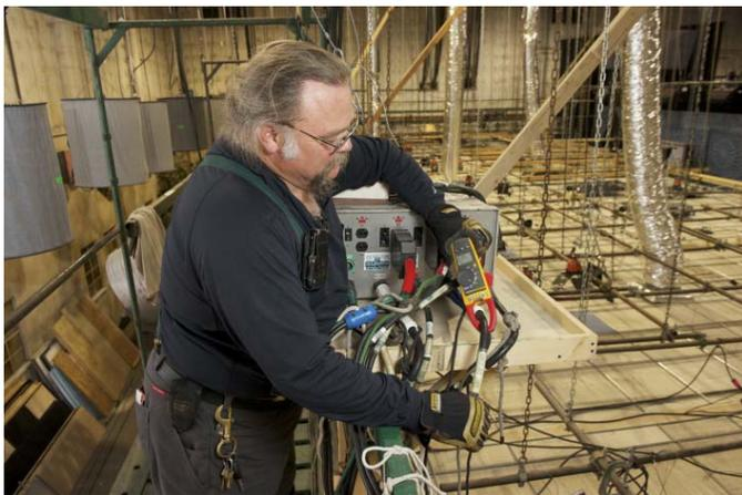
On a set for television production at CBS Studios, Roger Lattin checks the current on an overhead power supply with his Fluke 376 Clamp Meter.
