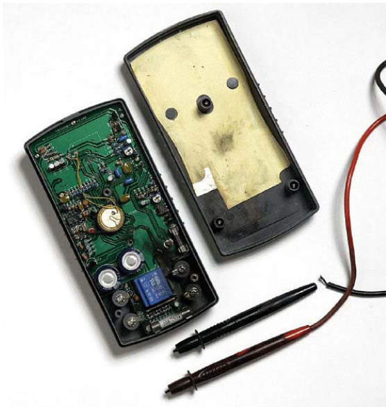
Failed digital multimeter and probes that were not certified by an independent rating agency.
