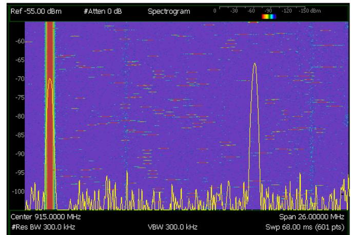
Figure 10. This shows a spectrogram display of a frequency hopping signal and a measurement sweep using the standard Clear/Write mode (yellow trace) superimposed over the spectrogram
