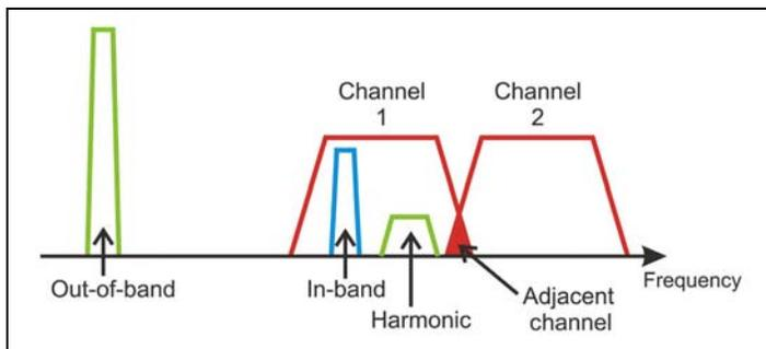
Figure 3. Diagram of several signals in a wireless environment resulting in different levels of interference occurring in Channel 1
