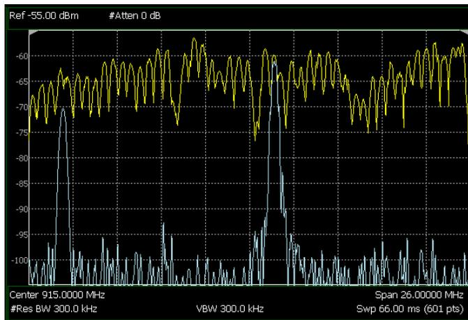
Figure 9. This screen shows the measurement of a frequency hopping signal as displayed in standard Clear/Write mode (blue trace) and MaxHold mode (yellow trace). It was observed that the signal to the left was stationary.
