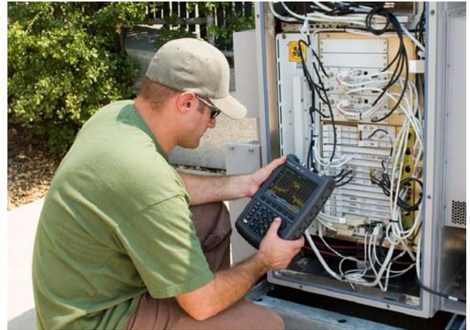
Figure 1b. FieldFox directly connected to a feeder line on a wireless communication system
