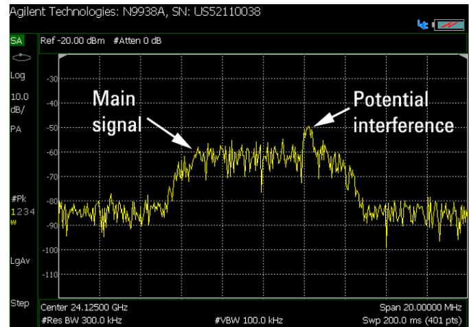
Figure 4. Measured spectrum of a 24 GHz microwave communications signal with lower-than-expected system performance and including potential in-band interference
