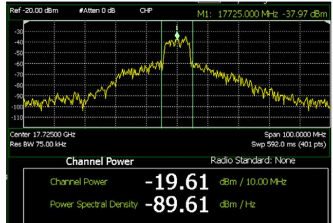
Figure 7a. Channel power measurement
