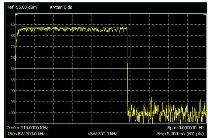
Figure 11. Measurement of a hopping carrier using the Zero Span mode on FieldFox
