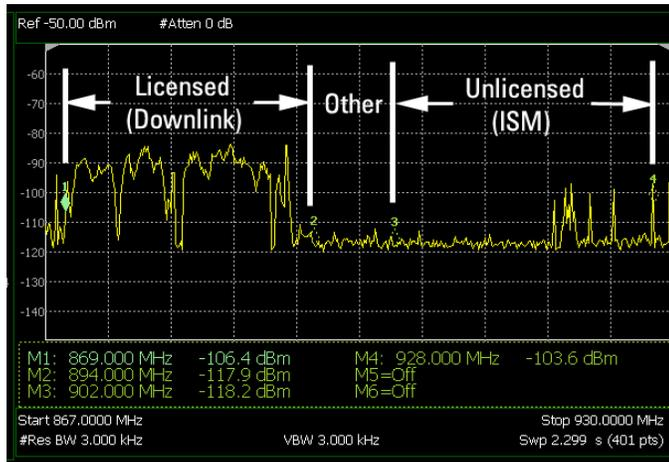
Figure 2. Over-the-air measurement of the UHF spectrum using FieldFox, showing a portion of the licensed cellular and unlicensed Industrial, Scientific and Medical (ISM) bands
