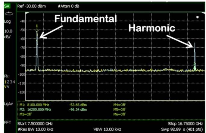
Figure 5. This screen shows the measurement of an 8.1 GHz radio communications signal being bandpass filtered (yellow trace) and left unfiltered (blue trace). The unfiltered response shows the observable second harmonic at 16.2 GHz.
