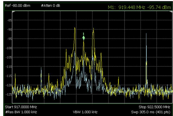
Figure 8. Over-the-air measurement comparing the received signal using an omnidirectional antenna (blue trace) and a high-gain antenna (yellow trace)
