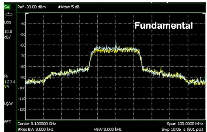
Figure 6a. Frequency response of the 8.1 GHz fundamental
