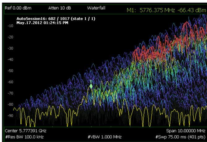
Figure 12. Waterfall display of a time varying signal
