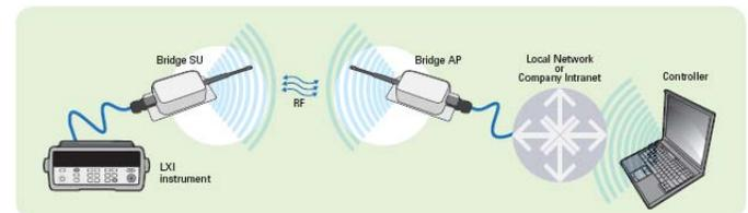
**Figure 1: Long-range Ethernet bridge setup**
