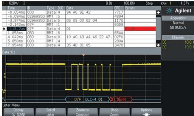
Figure 2: Hardware-based decoding captures and displays an infrequent CAN error frame that other scopes miss.
