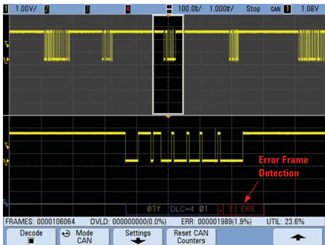
Figure 7. Agilent's MS07104A reliably captures and decodes CAN error frames using hardware-based decoding.
