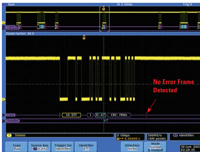
Figure 8. Tek's MSO4104A fails to capture and decode CAN error frames with a software-based decoding update rate of just one 1 decode every 5 seconds.
