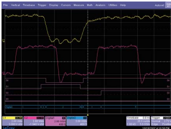
Figure 5. The LeCroy WaveRunner 104Xi – MS500 fails to capture the infrequent metastable state after 5 seconds of observation time.
