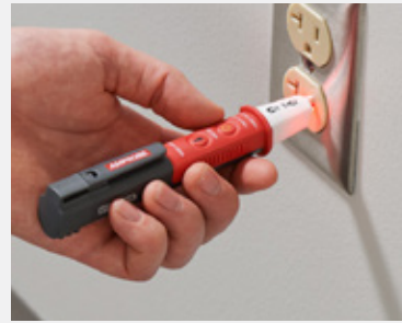
Test wall sockets for AC voltage
