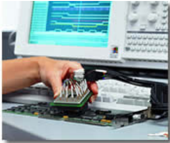
IC Test Clips are the ideal solution for probing dozens of leads on an IC chip and allow reliable connection without damaging the chip.
