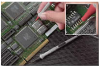
Pomona Electronics' Precision Electronic Probe features a pogo pin style tip of only 0.018" diameter for probing extremely fine pitch IC leads found in TSSOP and SSOP packages and densely populated circuit boards.
